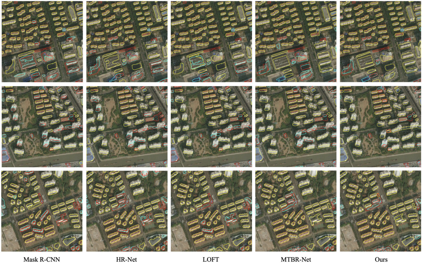
Fig. 8. Examples of building footprint segmentation results of different methods on the BONAI Shanghai test dataset. The yellow, cyan, and red polygons denote the TP, FP, and FN, respectively. Our method produces much more accurate footprint boundaries compared with other methods.
